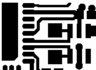
Figure 7. Layer 1 except showing the balun routes
