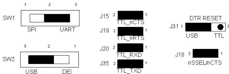
Figure 7. Jumper settings for RS-232 serial communication
