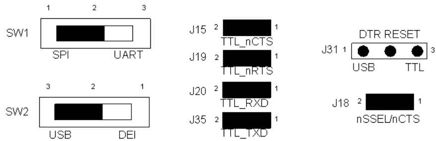
Figure 4. Jumper settings for SPI-mode USB RS-232 serial communication
